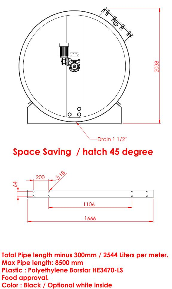
Dimensions: 1800mm inside 1950mm Outside Agitator: °sn/min 7 Motor 0,75kw 3x400 50/60hz
